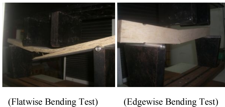
Figure 11. Condition of sample damage in bending test of LVL
