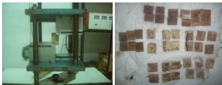
Figure 8. Condition of sample damage in the test of LVL shear strength.
