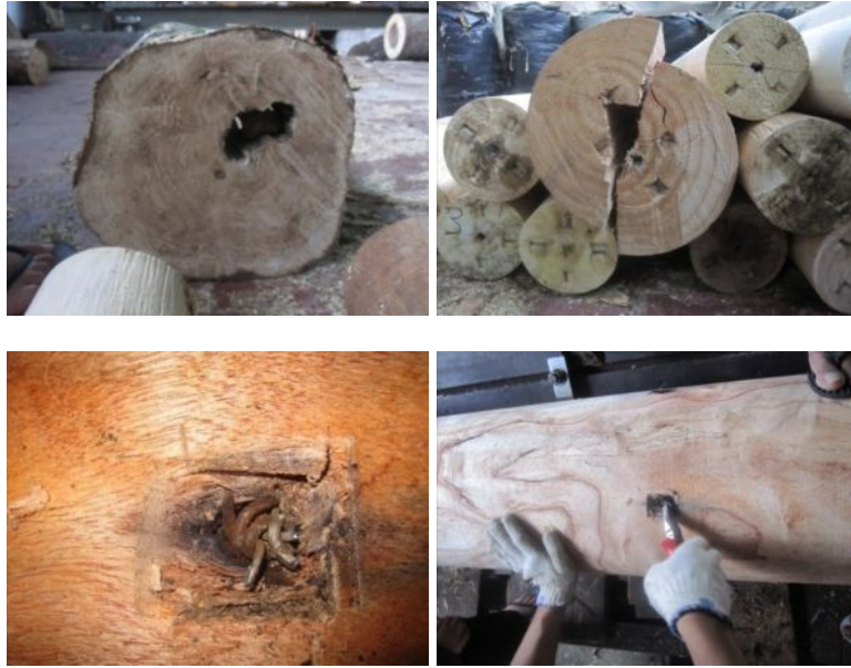
Figure 2. Physical condition of small diameter wood stems which were used as raw materials of LVL
